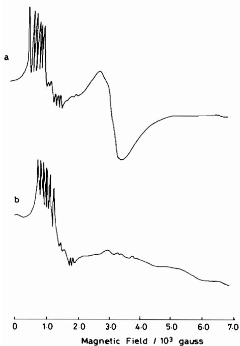
Fig. 7. X-band ESR spectra of (a) \text{MnBr}_2(\text{CNBu}^t) + \text{PBu}_3^n and (b) \text{MnBr}_2(\text{PBu}_3^n) in frozen THF, 93 K.
